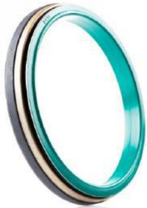
PTFE-lip cassette seal for crankshaft 0.5 bar pressure differential, 30 m/s rotational speed -35/+150°C temperature range
